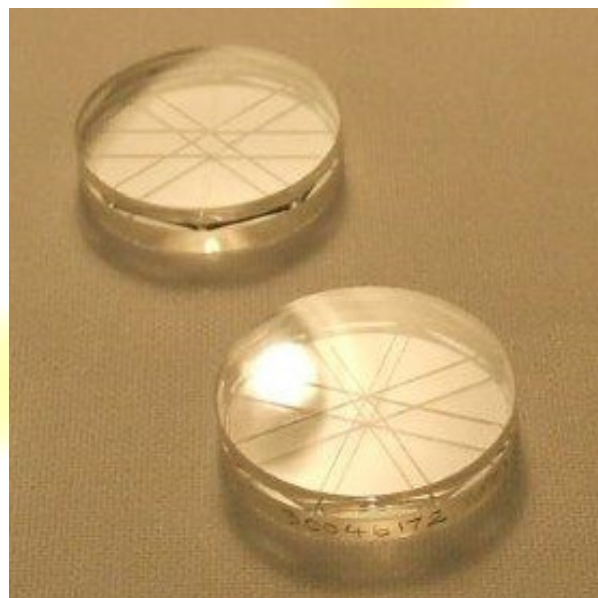
Fig. 7: G&H segmented waveplate prototypes
